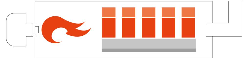
The high-tech ceramic Accuramics system is heated by the flame energy while the burner is running.
